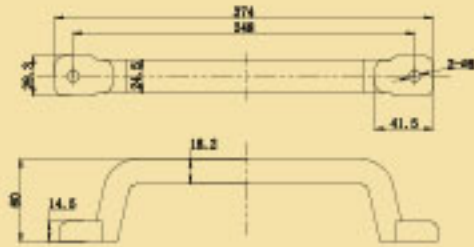
Rubber Handle Inside Steel
