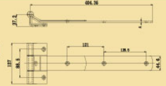
Strap Hinge Zinc Plated Steel
