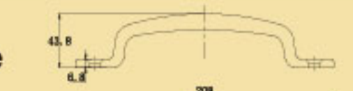
Die Cast Handle Chrome Plated Zinc Alloy
