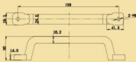
Rubber Handle Inside Steel
