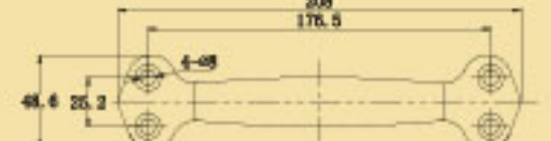
Die Cast Handle Chrome Plated Zinc Alloy
